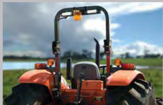
Typical Installation showing bar clamped to ROPS.
